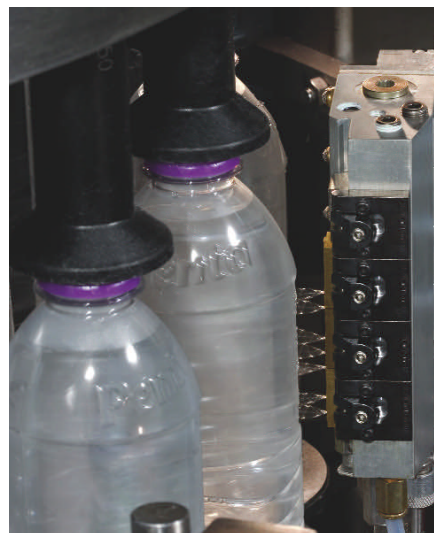
Non-contact wraparound labeling system accurately applies adhesive to containers.
