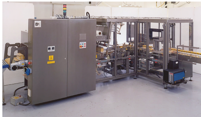
The all-in-one carton collation, tray-forming and shrink-wrapping system, above, saves valuable floorspace. At right, Keith Darroch, Twinings project engineering manager, left, and Europack sales director Ivan Reeve hold two of the eight possible package formats.
