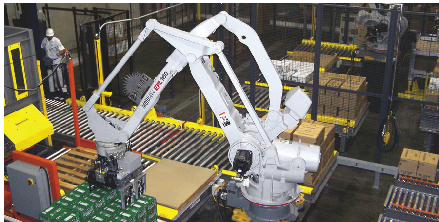
The robots stack product onto four-way wooden pallets in a multitude of different patterns. The robots also handle tier sheets and top sheets.
