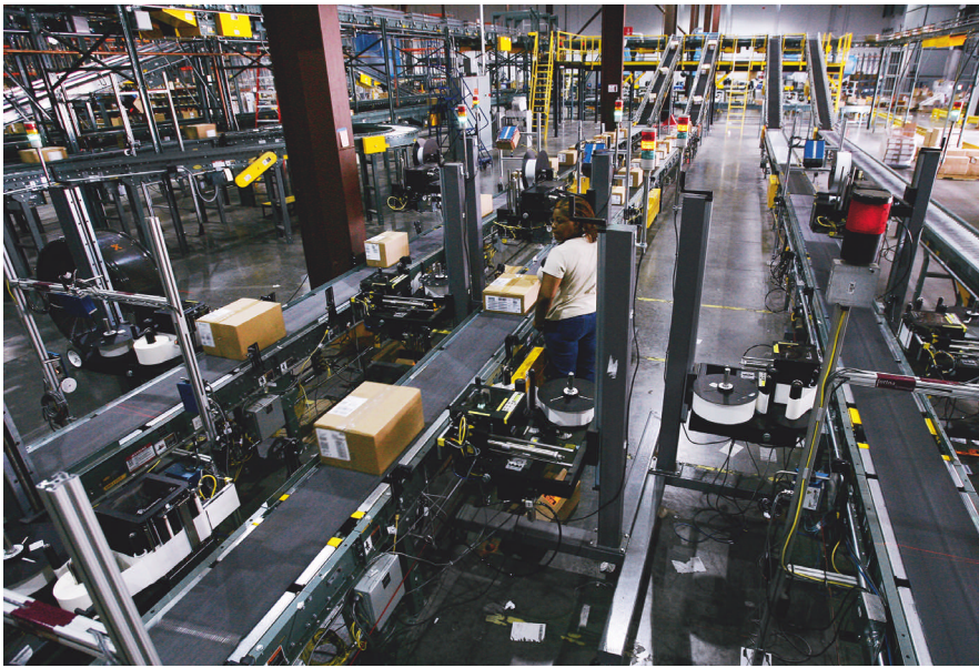
An overview shot of the RFID conveyor lines at Cingular Wireless in Memphis, above, shows three RFID print-and-apply case-conveying lines that together run 45 cpm.
