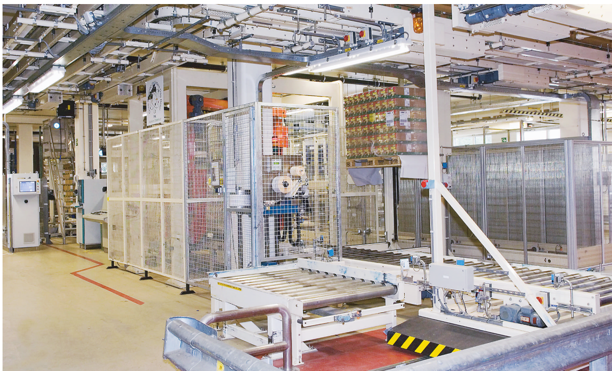
Three label printer/applifiers are in place in the caged area of Knorr's palletizing area, above. They're integrated with SAP using specialized software, so that Knorr can download production orders to create unique SSCC codes for pallets.
